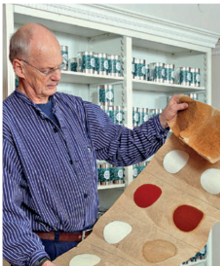
Paint on absorbent surfaces! One simple test to check the penetration and protective abilities of the paint/oil.
