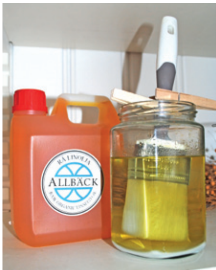
Keep brushes hanging in a jar with raw linseed oil. This oil can be used for impregnation.
